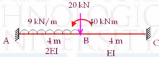
6. Find all the joint displacements for the beam in Figure 5, using direct stiffness method.
