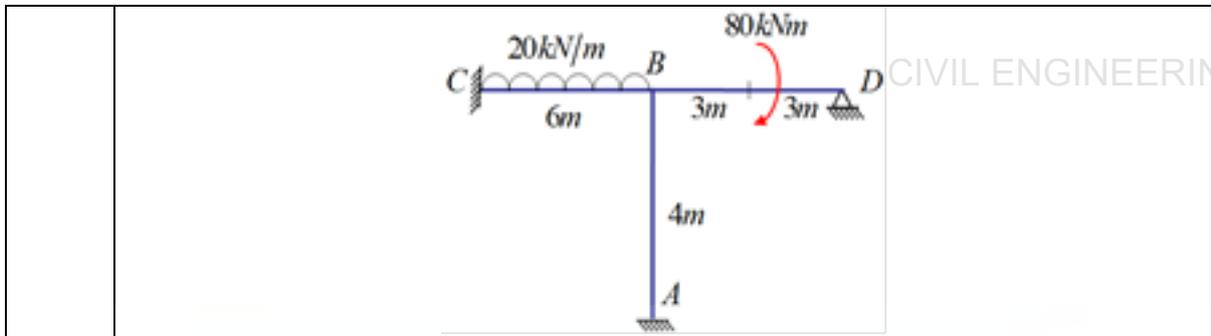
5. Determine the displacements at B for the beam shown in figure, using stiffness method.
